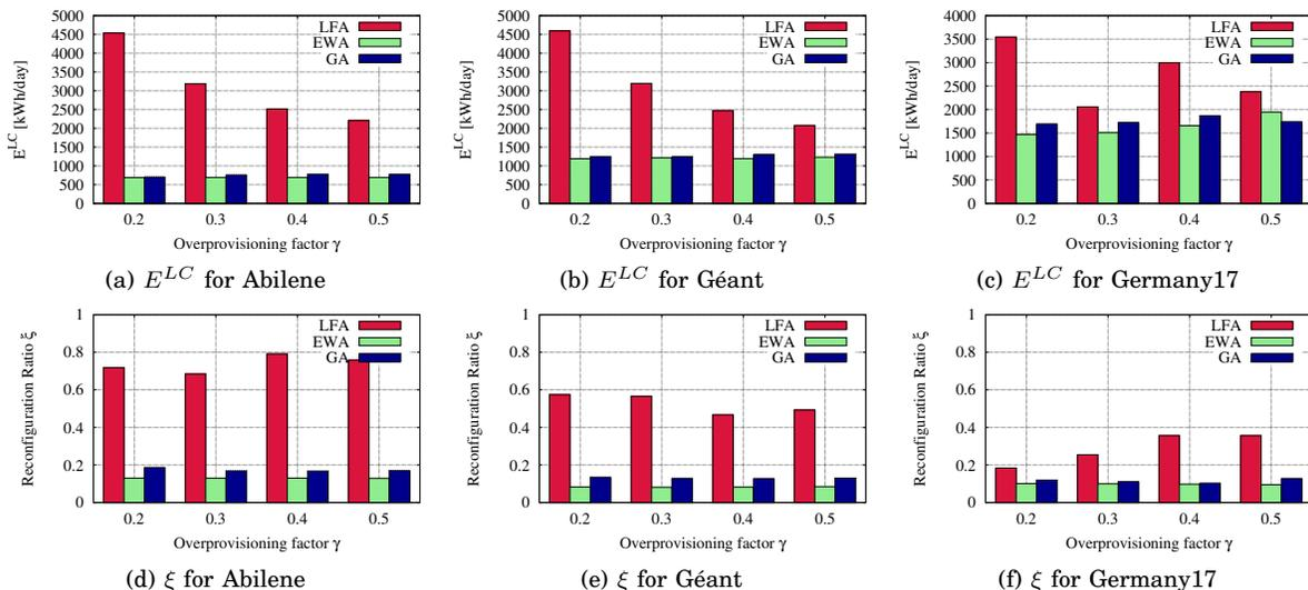
Fig. 6. SBN Variation: Energy consumption and reconfiguration ratio in the Abilene and Géant networks.
