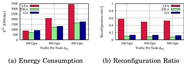
Fig. 8. Load Variation: Energy consumption and reconfiguration ratio in the Géant network.
