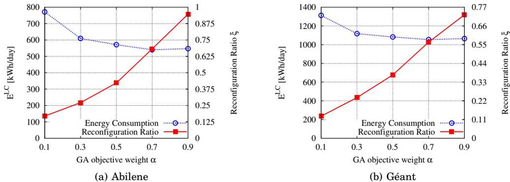
Fig. 12. GA Sensitivity Analysis for the Abilene and Géant networks.
