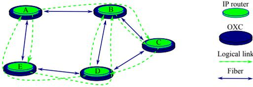
Fig. 2. Network model on exemplary logical and physical topologies.
