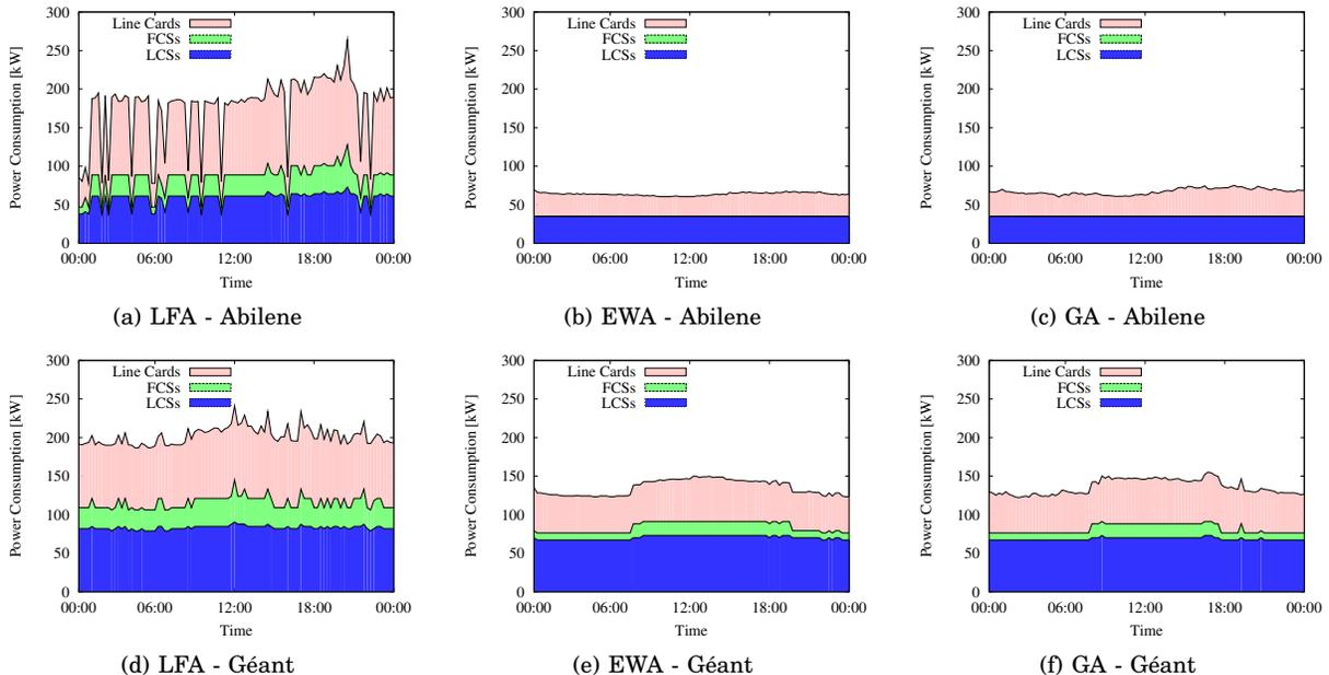
Fig. 13. Power Breakdown for the Abilene and Géant networks.
