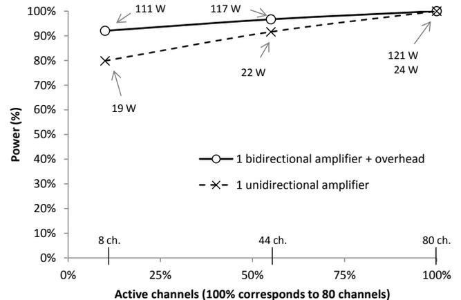
Fig. 8. OLA: power scaling with active channels
