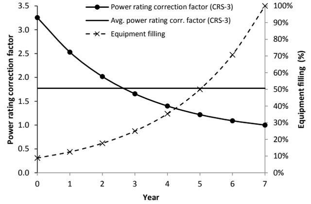
Fig. 2. IP router: CRS-3 power rating correction factor (left axis) and relative equipment filling (right axis) evolution over time.
